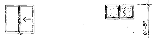
ALUM. SLIDER W/ INSUL. GLASS, SCREEN (SINGLE GLAZING) • LAUNDRY ALUM. SLIDER W/ INSUL. GLASS, SCREEN (OBSCURE GLAZING)
