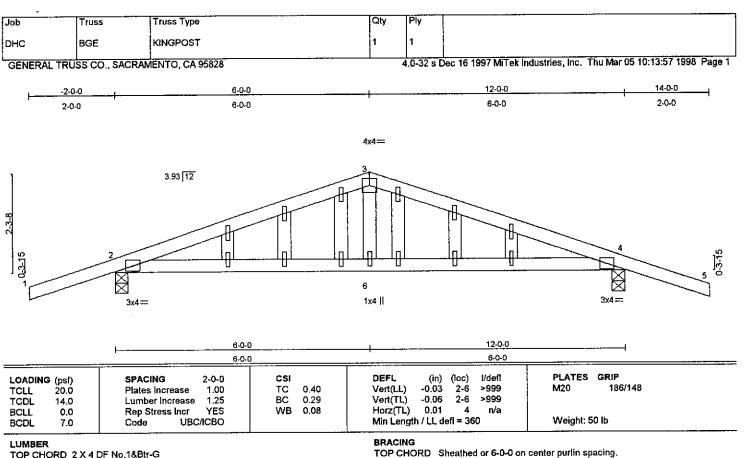
BOT CHORD Rigid ceiling directly applied or 10-0-0 on center bracing.
