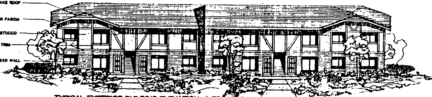
TYPICAL EXTERIOR BUILDING ELEVATION / FRONT & REAR SCALE 1/8"=1'-0"
