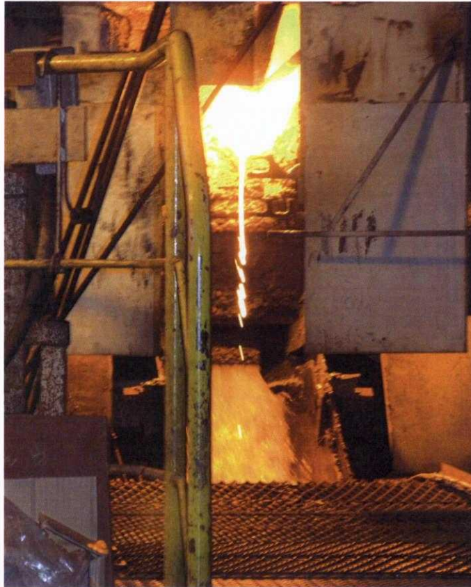
Figure 4 Molten slag from chamber (Photo courtesy of John Howard III)
