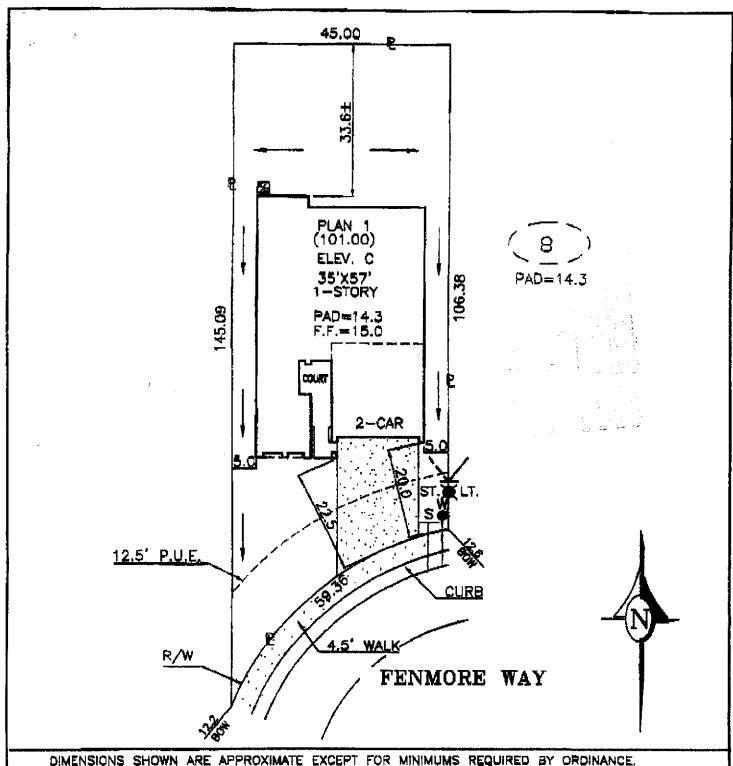
DIMENSIONS SHOWN ARE APPROXIMATE EXCEPT FOR MINIMUMS REQUIRED BY ORDINANCE. THIS PLOT DOES NOT REFLECT AS BUILT CONDITIONS AND MAY VARY FROM THIS PLAN.
